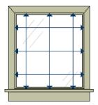
Measurement for <u>Inside</u> Mounted Blinds: Measure the inside width of the window casing in 3 locations and choose the smallest measurement. Then <u>deduct ½" from this measurement when ordering your blinds WIDTH</u>. For the Height simply measure the inside height of your window and order the exact height measured for the inside measurement.
