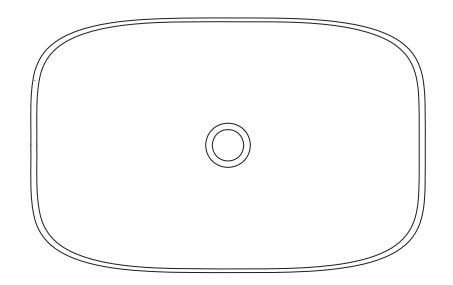
ALL DIMENSIONS ARE APPROXIMATE (+/- 1/2") AND ARE FOR REFERENCE ONLY. THE ACTUAL SINK MUST BE USED FOR CUT TEMPLATE AND/OR HOLE PLACEMENT.
