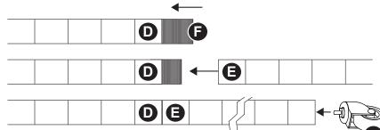
STEP 3. Slide poles with plastic cap on top through shelf corners until shelf rests firmly on sleeves. Push or gently tap the shelf down at corners to level shelf. Repeat steps 2 and 3 for each additional shelf.
