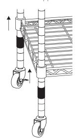
STEP 2. Starting at the bottom (the end with the small threaded hole and wheel), snap two sleeves (A) onto poles at desired intervals. The sleeves are marked with a directional arrow to show proper placement. Use grooves on poles to ensure even shelf placement among the four poles. NOTE: Place only enough sleeves to assemble bottom shelf. This step will be repeated for each additional shelf.
