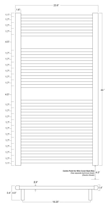
Position mounting brakets as near to each edge as possible and between the first or second cross bars
