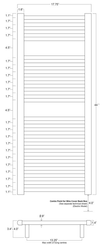
Position mounting brakets as near to each edge as possible and between the first or second cross bars
