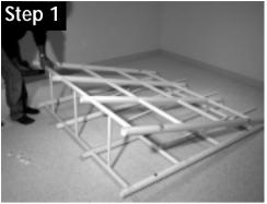
Insert Bottom Sliderails (**#8**) into Front Grid Assembly and fasten (*making sure fully inserted*) using 3- #08 x 3/4" Fastening Screws (**#1**) *Note: Fasteners in Bottom Hole Only*
