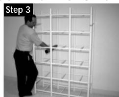
Fasten All Verticals to Horizontals Making sure all joints are pressed firmly together and tight against alignment dimples using 48 - #06 x 1/2" Fastening Screws (#1) Note: Fasteners in Holes Facing YOU Only-
