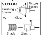
**Style#2** - Install proper bulb type and wattage. Remove the finishing screws that are already on your fixture. Position glass in place and secure with finishing screws.
