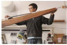
Stand the assembled body up and place the aluminum boom into the slot in the top of the body.
