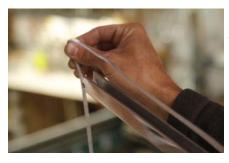
Drape the light engine cable over the roller at the end of the boom.
