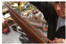
Once the boom is in the desired location, attach it using the two #8 wood screws.
