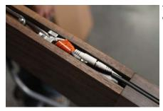
Tuck the connector and any extra wire into the groove.
