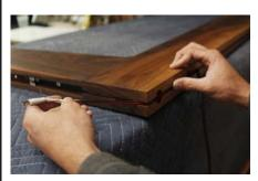
Place the wire in the groove, making sure it is laying flat and is not twisted.
