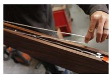
Adjust the height that the light engine hangs at by winding the cable around the studs in the groove in the top of the body.
