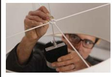
Place the cable through the slot in the shade spider.
