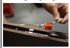
Place the knot in the light engine cable into the strain relief clip in the groove on top of the body.
