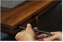
Once the joint has closed evenly, tighten the screws.
