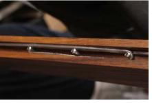
By wrapping the cable around different studs, the height that the light engine hangs at can be adjusted in 8 inch increments.
