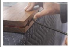
Press the rubber cord into the groove to neatly cover the wire.
