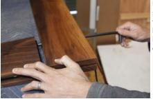
Insert the two 5" long 1/2-13 socket head cap screws into the holes and slowly tighten both screws using a 3/8" hex key. Assure that the joint closes evenly.
