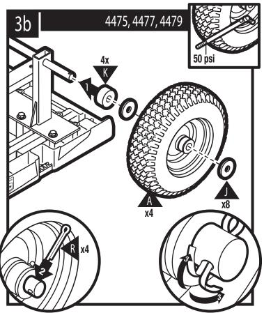
If unit is intended to be towed by a motorized vehicle, apply grease directly to both axle and wheel.
