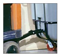
Tow hitch enables towing by a lift or fork truck; provided hitch pin allows multiple truck towing.
