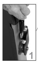
Insert the cable anchor lock through the activity bay opening and around the pulley so the anchor lock comes out and extends toward the anchor assembly at the center of the chair. For the top activity bay, insert the cable from the top. For the bottom activity bay, insert the cable from the bottom.
