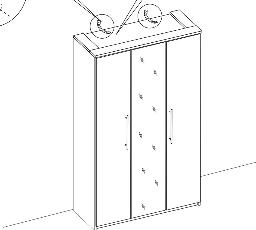
Wall fixings are not supplied with this product as different wall materials require different types of fixing devices( such as Rawl plugs used on brick work).You must use fixing devices suitable for the type of wall you intend to mount this product to. Please ensure that the head of any screw used has a diameter greater than the diameter of the mounting hole on the product and that the fixing is safe and secure before use.
