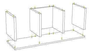
3 Start with the bottom horizontal zBoard (there will be holes on only one side of board). Align vertical zBoards to holes in the horizontal zBoard.
