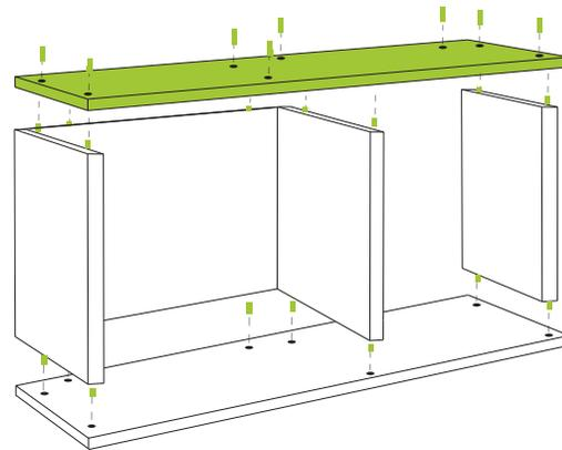
**3** Start with the bottom horizontal zBoard (there will be holes on only one side of board). Align vertical zBoards to holes in the horizontal zBoard.
