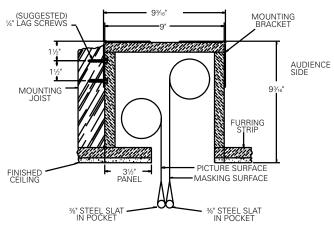
Offset mounting, recessed above ceiling. May be adapted for 1/4" paneling for ceiling.
