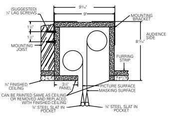
Offset mounting, recessed above ceiling. For plaster, dry wall, tile or paneling. Bottom of case painted same finish as ceiling.
