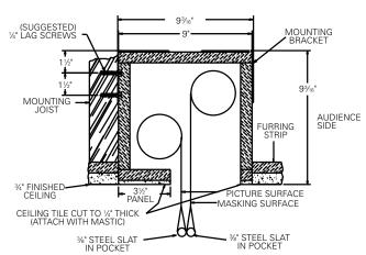
Offset mounting, recessed above ceiling. May be adapted for  $^3\!4"$  ceiling, but cut to  $^1\!\!4"$  thick under screen case and panel.
