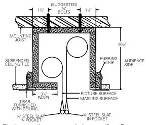
Flush mounting, recessed above ceiling. For use with dropped ceiling. May also be adapted for use with acoustical or other ceiling  $\frac{3}{4}$ " thick but cut to  $\frac{1}{4}$ " thick under screen case and panel.
