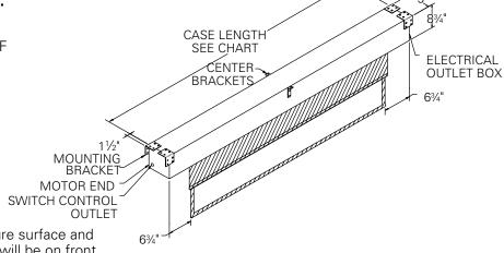
**NOTE:** Drawings below show picture surface and mask in the down position. Mask will be on front side of roller when retracted.
