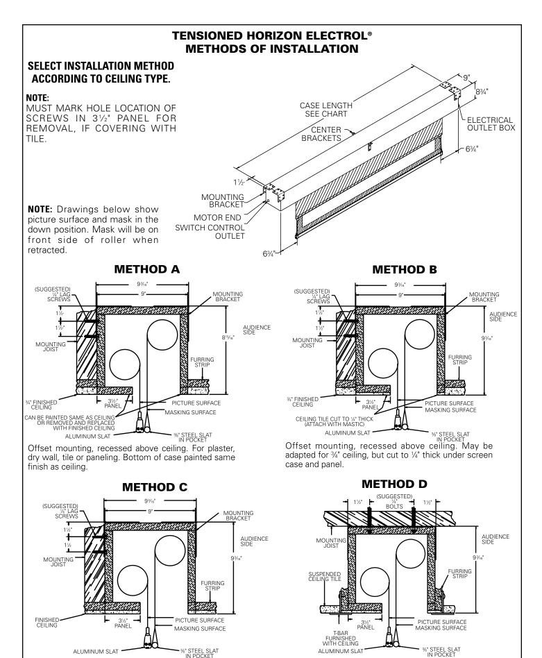
Offset mounting, recessed above ceiling. May be adapted for 1/4" paneling for ceiling.
