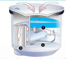
The cartridge acts as a funnel directing flow through the liquid sealant ①, preventing any odors from escaping. Next, the cartridge collects sediment ②, allowing the remaining waste to pass freely down the drain ③.
