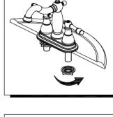
2. Place new faucet in position on sink. From under sink, thread mounting nuts onto faucet. Tighten mounting nuts.
