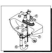
5. Apply a small bead of Plumber's putty to underside of flange (1). Insert body (2) into sink. Screw flange (1) into body (2). Pivot (3) must face faucet. Pull assembly down firmly and hold in place. DO NOT TWIST. Tighten nut, washer & gasket (4), clean off excess Plumber's putty
