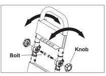
**STEP 2:** Attach the handle to the frame. Align holes, insert one 3/8" bolt and tighten the knob on each side. Adjust handle at the desired position.
