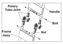
**STEP 1:** Insert rotary joints into handle and frame tubes so that stops point away from engine. fix them using 1/4" bolts and nuts on each side and tighten.
