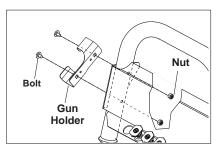
**STEP 3:** Use the carriage bolts to attach the wand holder.
