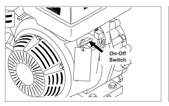
**STEP 8:** Turn the engine switch to "On" position. On Vanguard engines, move the throttle lever to "Fast" position, shown on the engine as a rabbit.
