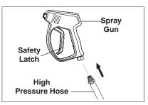
**STEP 5:** Attach the high pressure hose to the spray gun using teflon tape on hose threads.
