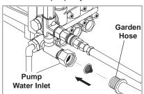
STEP 11: Check inlets filters, remove debris, then connect the garden hose to pump water inlet. CAUTION: Do not run the pump without water or pump damage will result.
