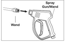
**STEP 6:** Attach wand to spray gun using teflon tape on wand threads.
