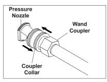
**STEP 8:** Release the coupler collar and push the nozzle until the collar clicks. Pull the nozzle to make sure it is seated properly.
