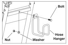
**STEP 4:** Use the 5/16" x 1" hex head bolt to attach the hose hanger.
