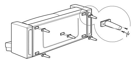
Finally, carefully lift and turn assembled unit onto its legs. Two persons required to avoid personal injury.
