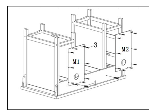
Connect the 1pc Right Back Panel (M1) and 1pc Left Back panel (M2) to the unit with 20pcs Wood Screw (3).
