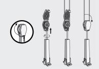
2. CEILING INSTALLATION. If rod is to be installed to ceiling, attach pulley housings (without brackets) and stirrup portion of center support directly to ceiling.
