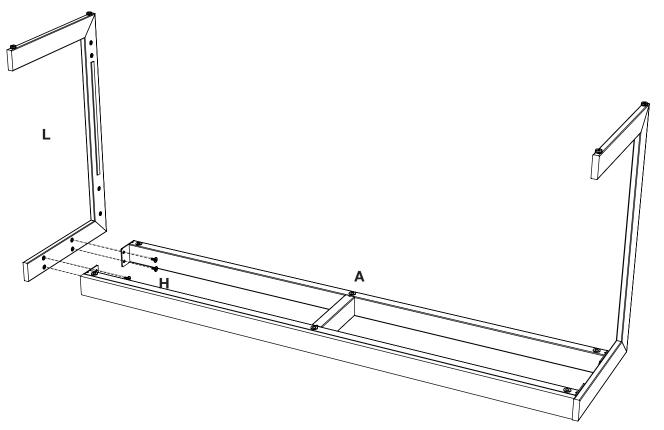
**Step 4**Attach **Upper Horizontal Beam (N)** to inside of Left and Right Leg using **Screw (H)** and **Hex Wrench (F).**
