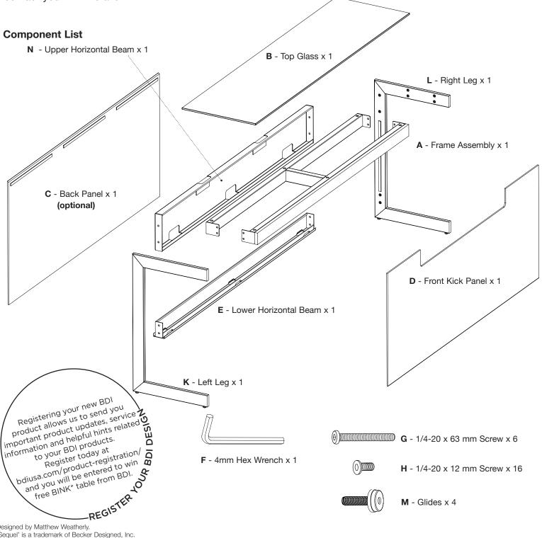
Step 1 Install Glides (M) to the bottom of Left Leg (K) and Right Leg (L).
