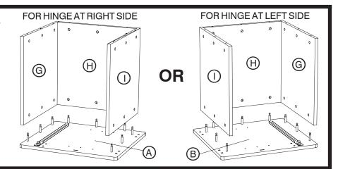
With the holes on its underside facing the front and bottom of the unit, insert the Wood Dowels of the L Half-Shelf into the holes in the Side Panel; tilt the Half-Shelf enough to insert the Bushings on the P Door into the hole in the Half-Shelf and the hole in the Bottom Panel. Straighten the Half-Shelf.
