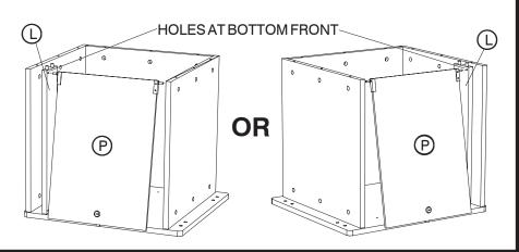
6 Slide the Screw Posts on the remaining Side Panel into the corresponding holes in the Top, Back and Bottom Panels (making sure that the Wood Dowels also engage), and lock all Cams.
