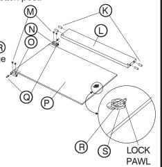
Depending on whether you want the Door to hinge on the left or on the right, select the Side Panel OPPOSITE the hinge side (both options are shown in this and the next two steps). Slide the Top, Back and Bottom Panels down onto the Screw Posts, and secure by turning each of the engaged cams clockwise until they stop.
