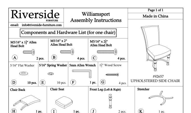
Be sure to check all packing material carefully for small parts, which may have come loose inside the carton during shipment. Separate, count and check all parts against the Components and Hardware List above. Failure to use the correct length bolts in the proper locations may result in an unsafe product and could also cause damage to the parts being assembled.
