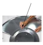
Next, align the sides of each outer piece and the center piece and insert the next 3 bolts through both holes. Tighten castle nuts on bolts.
