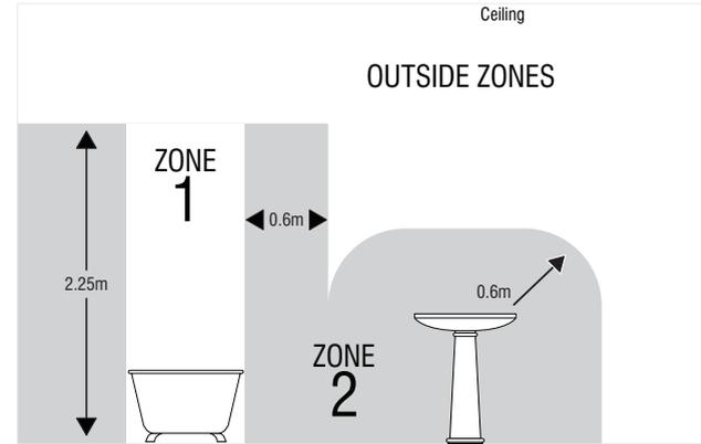
This product is suitable for use in Zone 1, Zone 2 and outside Zones of a bathroom. See diagram. If this unit is being fitted in a room containing a bath or shower, a 30mA RCD must be used - in accordance with IEE regulations.
