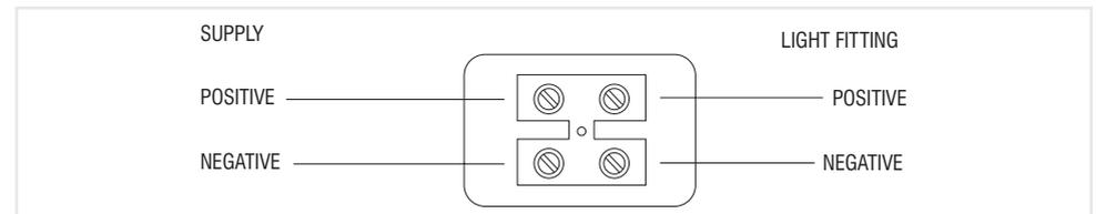
Connect the mains supply wiring to the transformer as detailed in the transformer instructions, ensuring that
