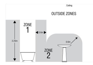
This product is suitable for use in Zone 1, Zone 2 and outside Zones of a bathroom. See diagram. If this unit is being fitted in a room containing a bath or shower, a 30mA RCD must be used - in accordance with IEE regulations.
