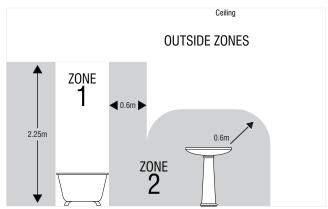
When used with the 42914 bezel, this product is suitable for use in Zone 1 and Zone 2. Other Bezels are outside Zones **ONLY** in a bathroom. See diagram.
