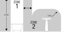
This product is suitable for use in Zone 2 and outside Zones of a bathroom. See diagram. If this unit is being fitted in a room containing a bath or shower, a 30mA RCD must be used, in accordance with IEE regulations.
