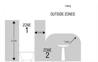
This product is suitable for use in Zone 2 and outside Zones of a bathroom. See diagram.
