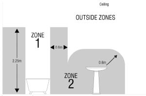
This product is suitable for use in Zone 1 and Zone 2 and outside Zones in a bathroom. See diagram. If this unit is being fitted in a room containing a bath or shower, a 30mA RCD must be used - in accordance with IEE regulations.
