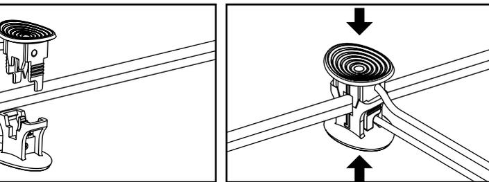
4.2 Align and fit the main low voltage cable vertically to the slot of wire connector as shown.
