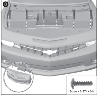
Fit front bumper onto the vehicle. Insert 6 screws and tighten.
