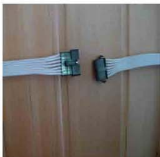
FIG-17 Link the control panel connectors
