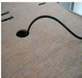
FIG-19 Slip the power plug through external top board
