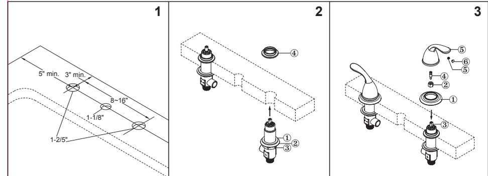
4. Place spout assembly (1) through mounting hole in deck. Secure spout with rubber washer (2), metal washer (3) and nut (4). Tighten nut (4) securely with wrench.
