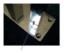
Attach the spout by pushing it over the brass spindle. Please make sure the grub screw is fully removed so the O rings do not become damaged. Line up the spout, and tighten grub screw. The mixer is now fully operational by using the handle.
