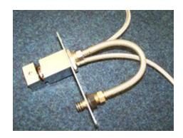
Attach the outlet/spout connection pipe to the connector from the back of the body to the spout thread using the ½" BSP flexible pipe. A loop must be made so the pipe can be pushed upwards or downwards into the wall recess.
