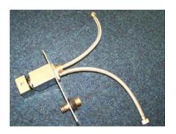
Attach in the flexible inlet pipes. Do not over tighten. These are to be plumbed into hot & cold water supplies. Flush out the pipes prior to this to remove any debris.
