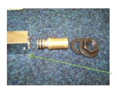
Remove the brass spindle from the spout by loosening grubscrew.
