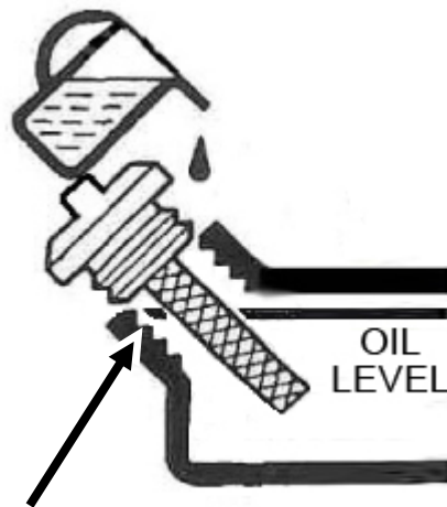
Figure 2 - Add Oil To TOP Of Threads
