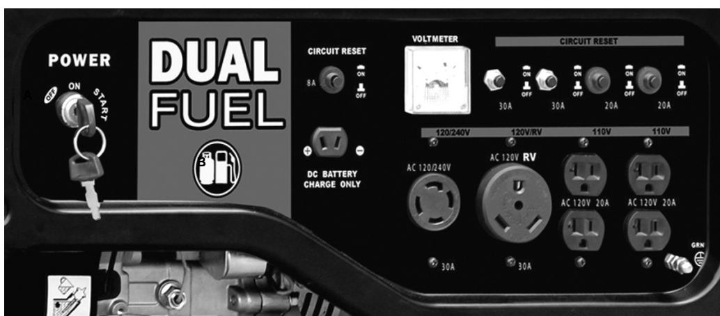
Figure 8 - Outlets available on this generator, from left to right: 12V DC, 120/240V AC, 120V AC RV, and 4 each 120V AC.
