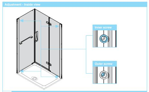
Adjustment screws are located on the stile profile at the top & bottom. Adjustment is made using the large & small allen keys. Adjustment is provided for each side.
