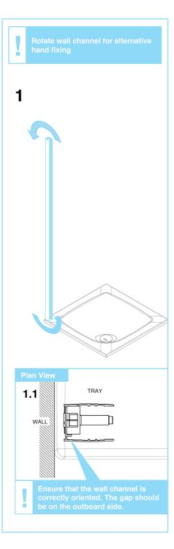
Rotate alternative hand fixing.
