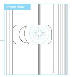
Lock the adjustment mechanism by fully tightening these screws.
