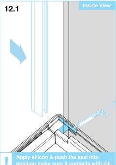
position make sure it contacts with o Remove any excess silicon.
