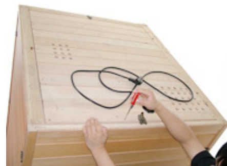
FIG-20 Fix the external board with screws
