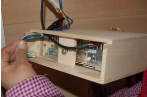
FIG-15 Link the CD connectors
