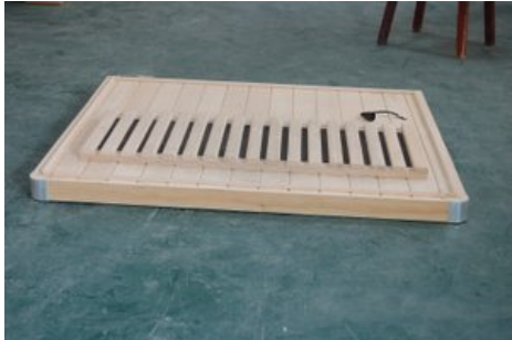
FIG-3 Placing bottom floor
