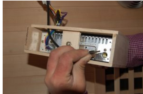
FIG-16 Link the antenna connectors
