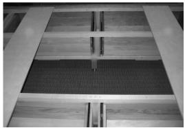
Attach a center support leg to the inside of each of the storage rails. Extend the leveler leg to contact the floor. (See image above)
