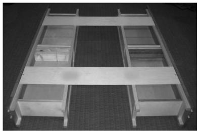
Attach 2 of the plywood deck pieces across the top near either end of the storage rails (See image above) using a  $#10 \times 1 \frac{1}{2}$  screw in the hole at the end of each piece. The remaining holes will not be utilized.
