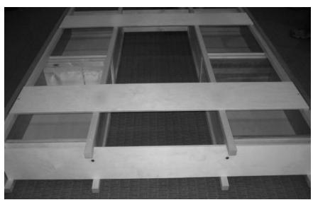
Attach the 2 vertical plywood ends to either end of the storage rails using 2 of Allen head machine screws supplied for each piece. (See image above)
