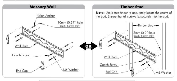
Tip: Use the built-in spirit level to ensure wall plate is horizontal
