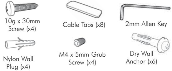
**Tools Required:** • Power drill • 4mm (3/16") drill bit • 6mm (1/4") drill bit • Phillips head screwdriver
