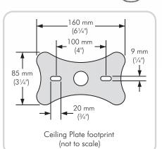
Maximum distance bracket can be secured from top of projector = 10 mm (3/8)
