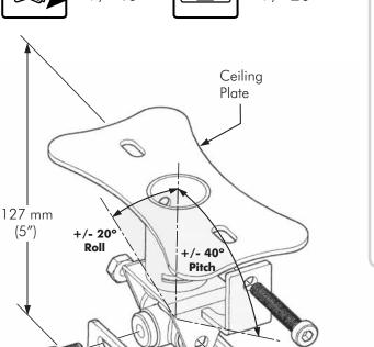
NOTE: 4 sets of Extension Bracket lengths are included to suit most mounting configurations. Any combination of these brackets may be used.
