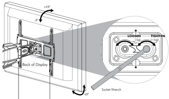
Position your display to the desired viewing angle, using the angular movement allowed by the double ball mount.
