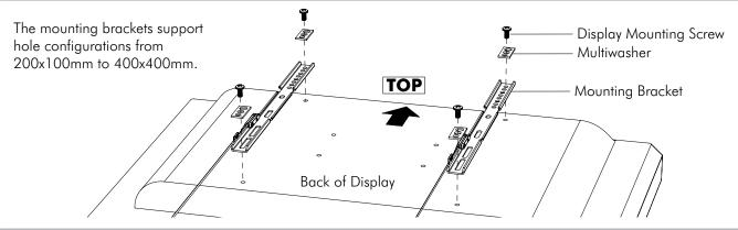
Step 5. Attaching/Detaching Display to the installed Arm (2 people required)
