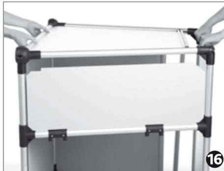
*Last add the left side panel. For this press all four corners down evenly and with force. It is normal that the transport box is under high tension for this step. This is necessary to prevent it rattling when you are driving later. If you cannot fit this last panel correctly, it might be helpful to loosen the pre-mounted screws of this panel at the corners.*
