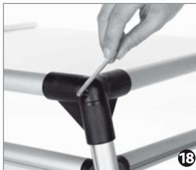
*Once all screws are tight and the box is fully assembled and straight and stable, loosen the screws in the upper corners and fit them in again with the protective caps.*
