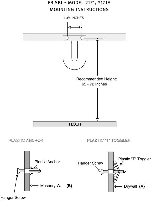
CAUTION : These instructions are intended for **drywall installation only**! If installation is to be other than drywall, the installer shall use appropriate hardware for the wall structure.
