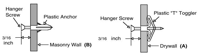
CAUTION: These instructions are intended for **drywall installation only**! If installation is to be other than drywall, the installer shall use appropriate hardware for the wall structure.
