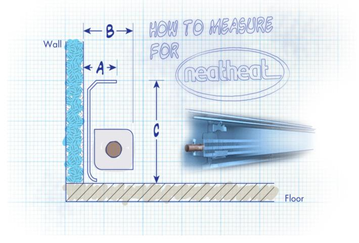
A = The measurement from the wall to the front edge of the metal enclosure attached to the wall. This measurement must be 2" or less.
